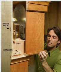
21 Slide the hood into position on top of the waist molding. Retaining blocks on the waist sides hold it in position. Fasten the hood to the back with brass hooks.
