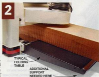
All folding extension tables need additional support to minimize snipe on long and heavy boards. Long tables are best, as shown above, but no planer has tables that are rock solid.
