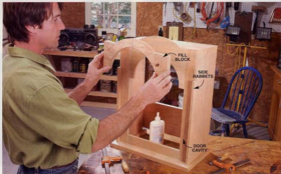
9 Installing the fill block completes the recess for the door and readies the hood for its arched cornice.
