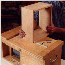
Sand surfaces flat and smooth in no time. The sanding drum is 18-in. wide, but this machine works best with boards that are less than 12-in. wide and 24-in. long. It's very effective for drawers and boxes, too.
