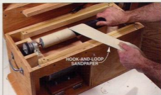
Changing sanding grits is easy. Just open the hinged lid, peel off a roll of reusable hook-and-loop paper and wrap a new grit.
