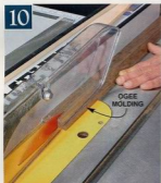
10 Rip the cove, ogee and beaded moldings to final width on your tablesaw. The cove molding gets ripped once to remove the waste portion while the boards for the ogee and beaded moldings get ripped twice.
